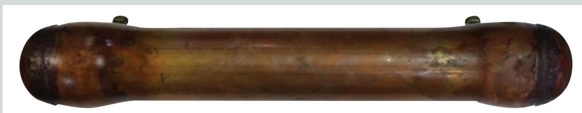
Figure 4.1b Sample after exposure to 7,500 kPa (6 times SWP)
