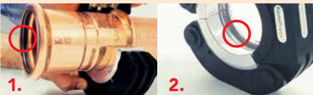
3. Ensure you have the correct sized fitting, check the fitting is clean and the stainless steel grip ring and O-ring are free from debris and correctly seated in the fitting.
